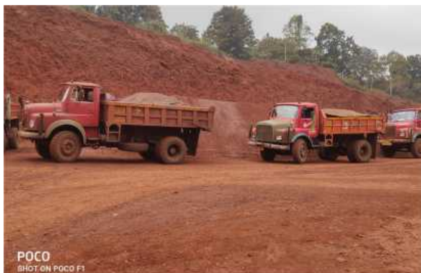
Photo-13: Mineral dispatch truck with tarpaulin cover on top
