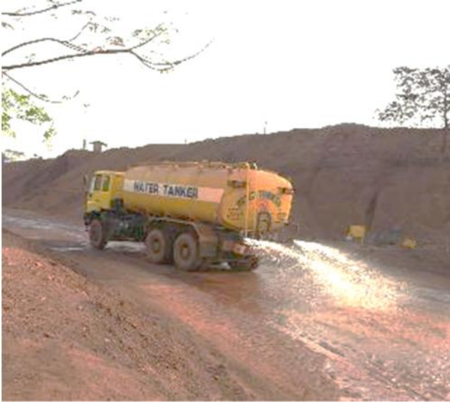
1. Mobile Water Tanker for dust suppression on mines haul roads.
