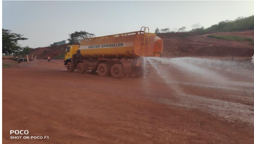
Mobile Water Tanker for dust suppression on mines haul road
