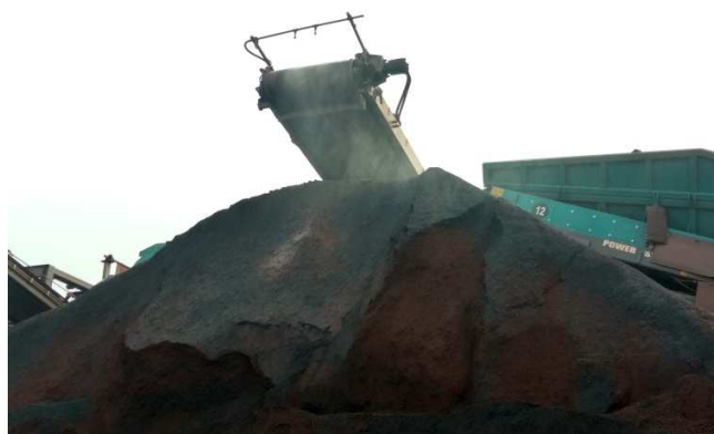
Dry fogging arrangement at mineral handling plant
