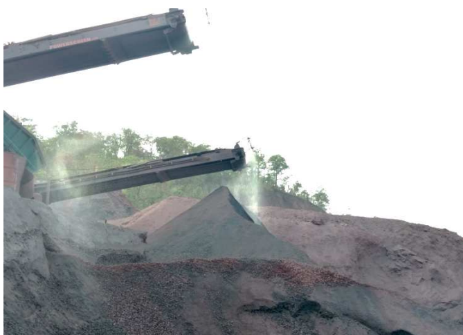
Dry fogging arrangement at mineral handling plant
